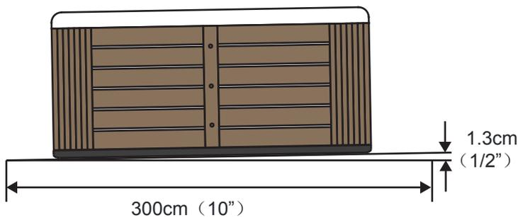
For correct water drainage, the inclination should be 1.3 cm (1/2 inch) / 305 cm (10 inches)
