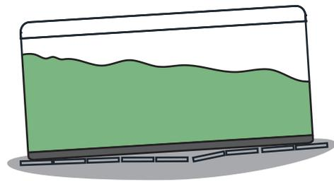
The spa could lose its leveling state because of the sinking of the stones or bricks
