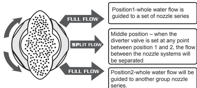
Important: when the diverter valve is in the "middle" position, from the design perspective of the spa, the nozzles can not provide the maximum pressure. However, when the diverter valve is in this position, you can turn the switch to close the unused nozzle, in order to increase the pressure of the selected nozzle.
